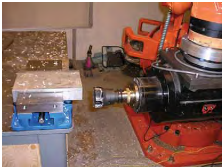
Figure 26. Robotic Milling Setup
