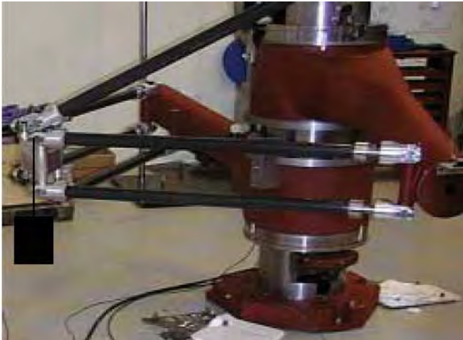
Figure 24. Setup of the TAU robot's Stiffness Measurement
