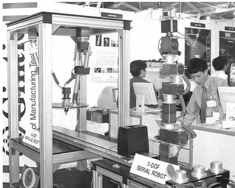
Figure 15. A light machining workcell with modular robot components
