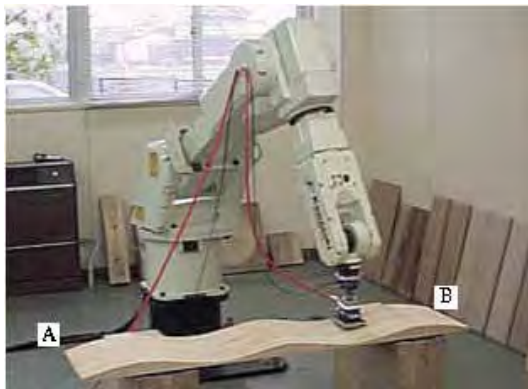
Photo 1. Robotic sanding system.
