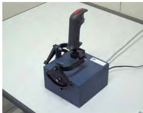
Photo 3. Joystick system used in teaching experiments (Impulse Engine2000).
