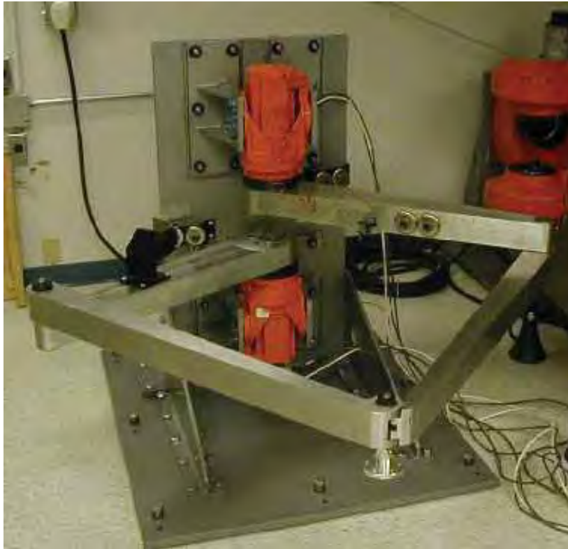
Figure 14. Two-Arm Test Platform (double SCARA structure)
