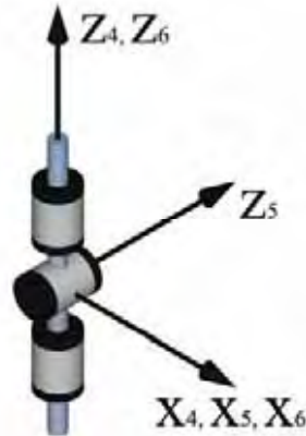
Figure 8. Zero-Displacement Diagram for the Roll-Pitch-Roll Spherical Wrist
